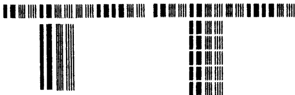
Illustration 14: Dot separation. This was printed on the dot matrix at 144 X 160 lines per inch. The lines are separated by 1, 2, 3, and 4 pixels from left to right.
